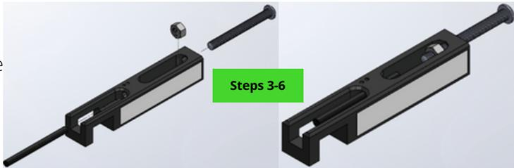
5. Insert *Bolt* into *Sight Pusher* as shown in step 4.
